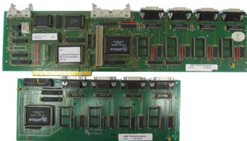
Figure 2-14: Datapath Card with Expansion Board
