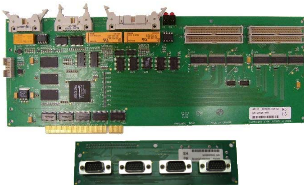
Figure 2-15: Image Accelerator Card with HeadIF Board
