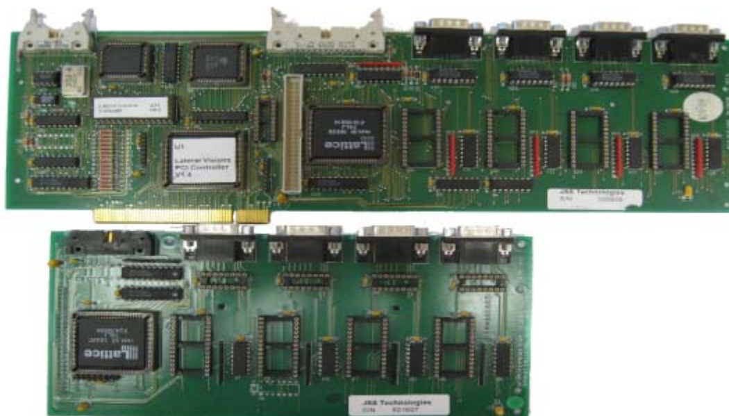
Figure 2-13: Datapath Card with Expansion Board
