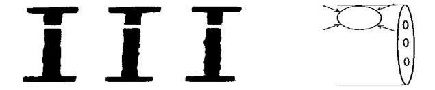
Figure 4.9 - Illustration of a print image demonstrating a missing channel due to an air bubble.
