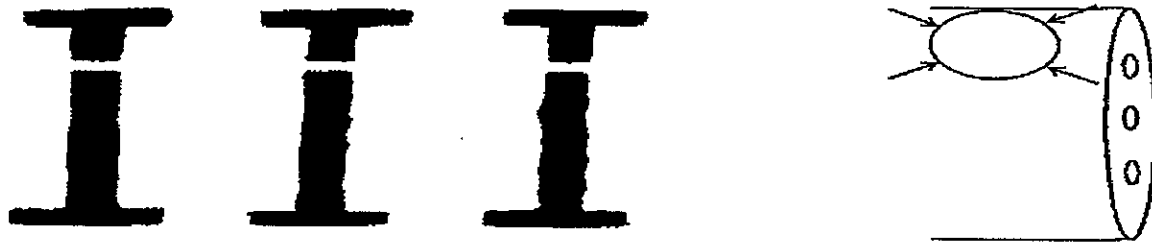
Figure 4.8 - Missing Channel due to an air bubble. 1
