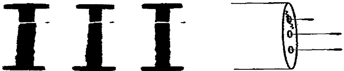
Figure 4.7 - Paper dust or debris in an orifice. 1
