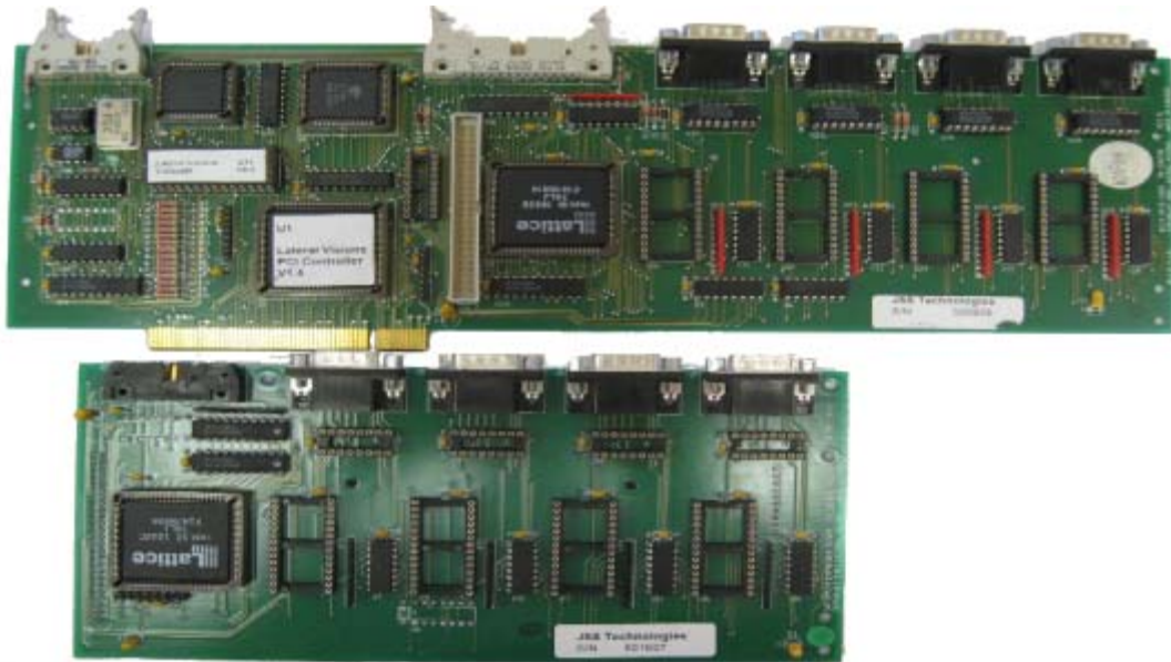
Figure 2-17: Datapath Card with Expansion Board
