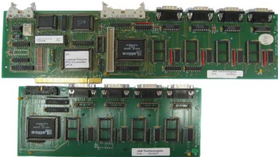
The Datapath Card supports four data connections for printheads. An expansion board is required to add support for an additional four data connections (for a maximum of eight printheads).
