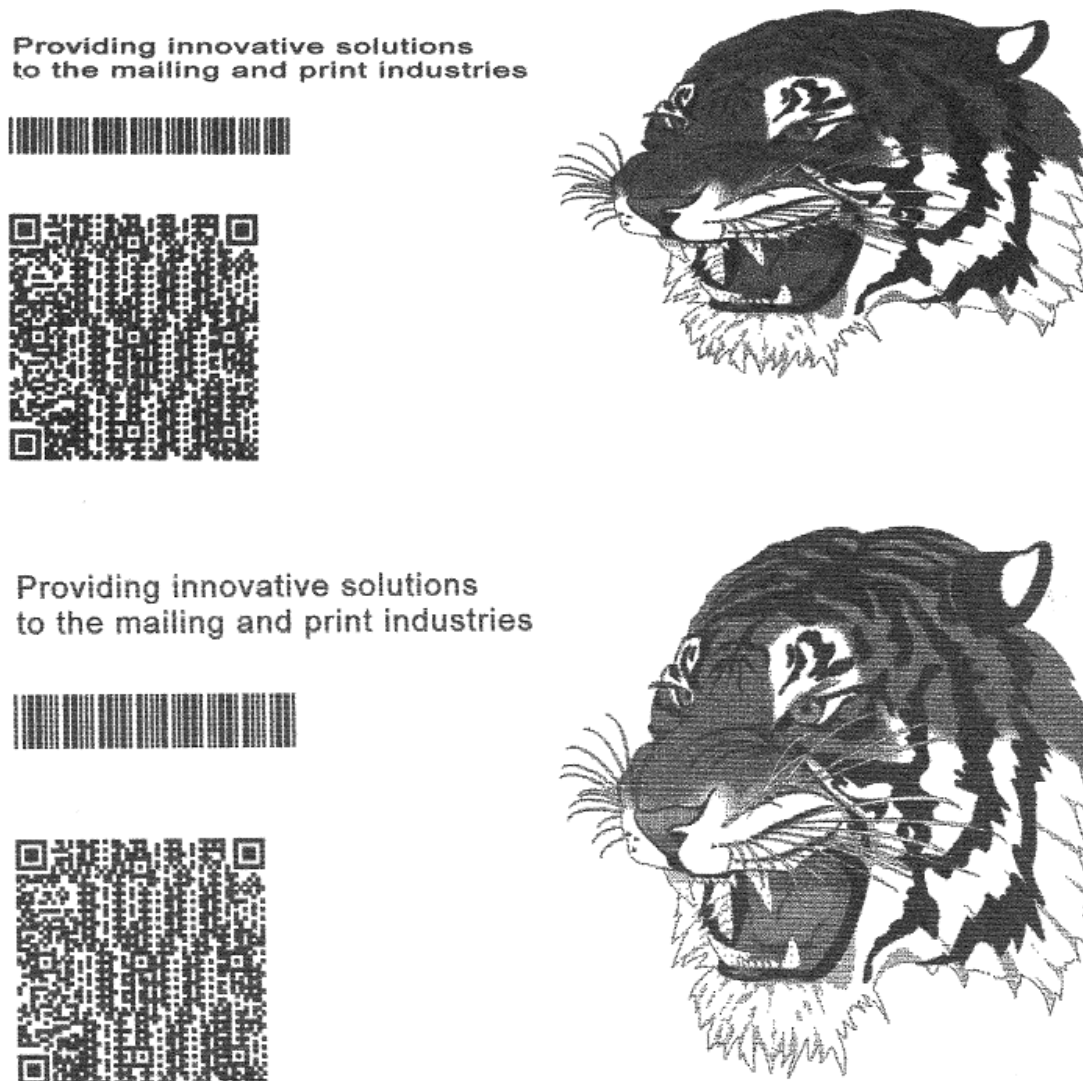
Figure 4-5: Compressed Image (Top) vs Normal Print (Bottom)
